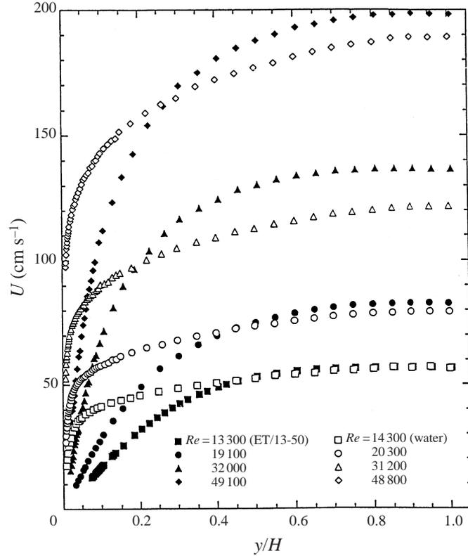
FIGURE 4. Mean streamwise velocity,  $U$ , versus normalized distance from the wall,  $y/H$ .
