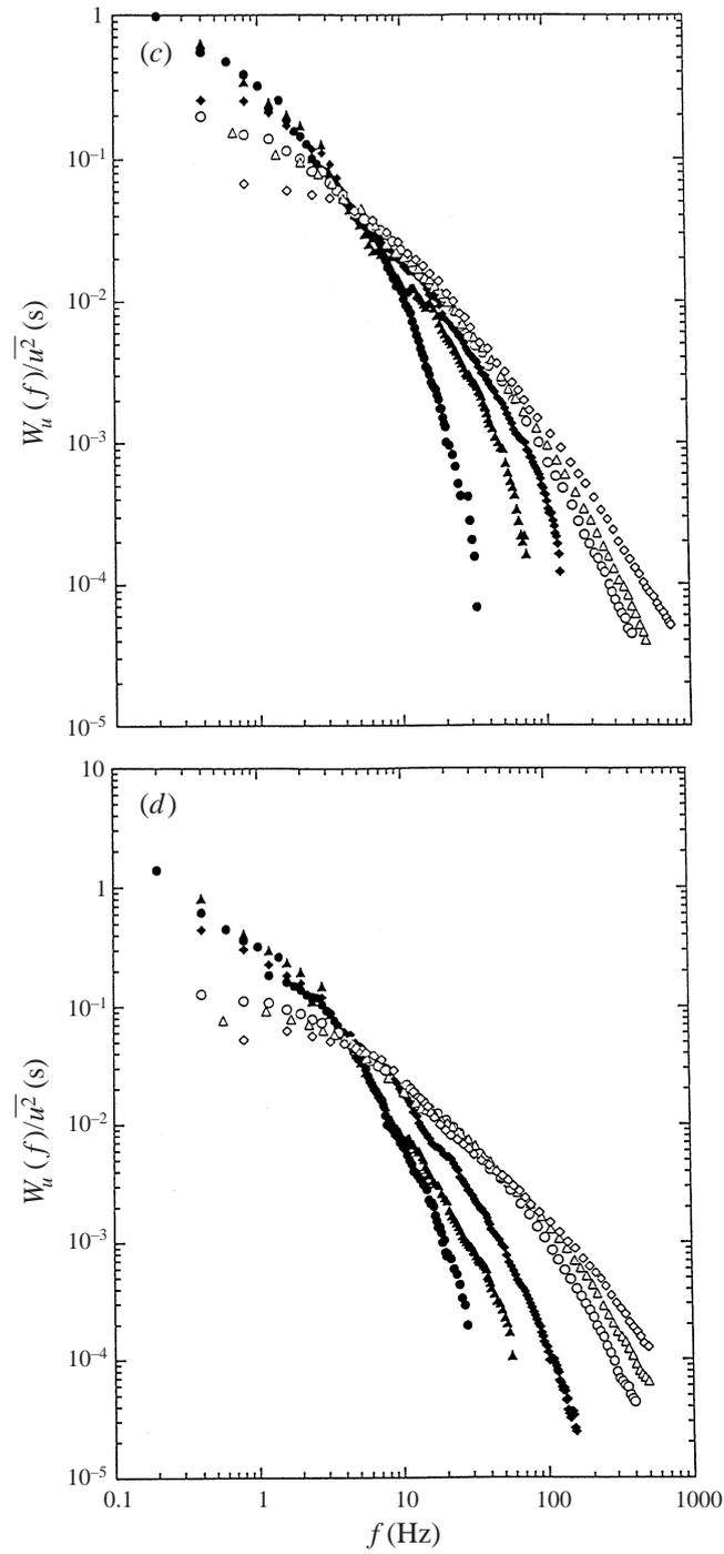
FIGURE 11. Streamwise velocity power spectra with the spectral density function normalized with the mean square of the velocity fluctuations, (a) at  $y/H = 1.0$ ; (b) at  $y/H = 0.6$ ; (c) at  $y/H = 0.4$ ; (d) at  $y/H = 0.1$ . ET/13-50:  $\bullet$ ,  $Re = 19\,100$ ;  $\blacktriangle$ ,  $32\,000$ ;  $\blacklozenge$ ,  $49\,100$ . Water:  $\circ$ ,  $Re = 20\,300$ ,  $\triangle$ ,  $31\,200$ ;  $\diamond$ ,  $48\,800$ .
