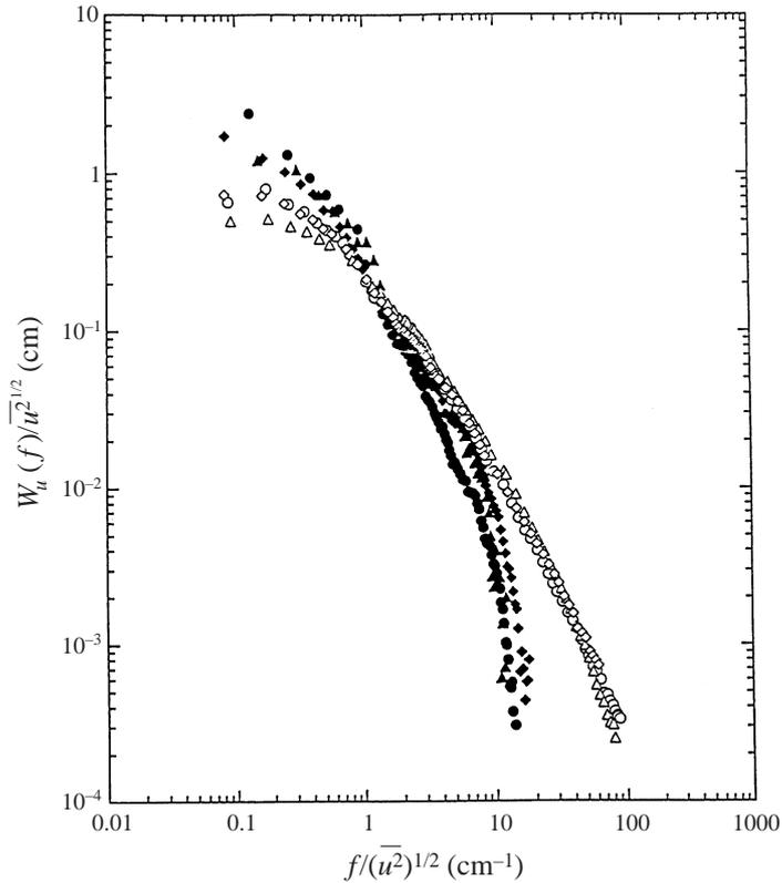
FIGURE 12. Streamwise velocity power spectra at  $y/H = 0.6$  with the spectral density function and frequency normalized by the root mean square of the velocity fluctuations. ET/13-50:  $\bullet$ ,  $Re = 19\,100$ ;  $\blacktriangle$ ,  $32\,000$ ;  $\blacklozenge$ ,  $49\,100$ . Water:  $\circ$ ,  $Re = 20\,300$ ,  $\triangle$ ,  $31\,200$ ;  $\diamond$ ,  $48\,800$ .
